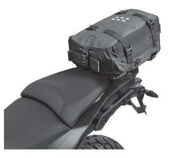
To fit, remove the KTM baggage carrier. Add thread lock to the 25mm M6 screws and insert from the underside.
