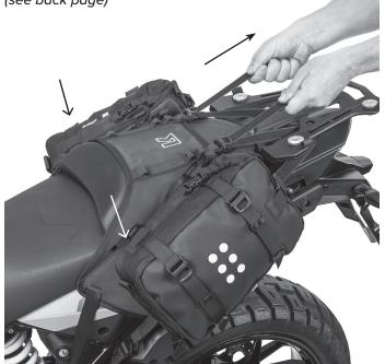
**3** Standing at the rear of the bike hold both loose straps ends and pull until the OS-BASE is firmly mounted on the seat. A strong tap downwards on each OS-PACK will help the OS-BASE slide further onto the seat.
