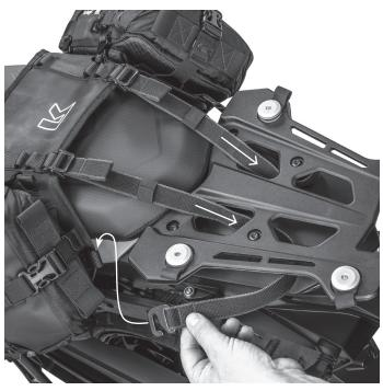
**2** Set the top straps to the longest length and slide the elastic loop near to the buckle. Pass a top strap down through the opening on the baggage carrier and around the rear alloy spacer and hook to the web loop, with the hook pointing down. Repeat on the other side.
